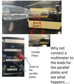
If electrons move through the gap from one plate to another, perhaps a measurable potential difference will develop between the plates. Multimeter is set to 200 mV range. When HeNe laser light is incident of plates...
